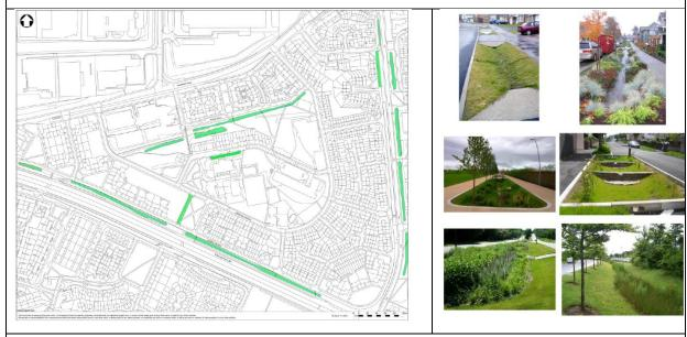
MM provided an overview of swales and how they can be provided with or without intermediate flow controls/dams depending on topography. Quite a few areas with large grass verges which could potentially be used for swales.
