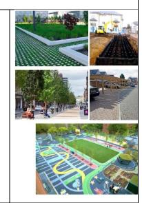
MM described that increased subbases or geocelluar can be used as attenuation storage in conjunction with permeable surfaces. Some areas identified which are currently parking areas.
